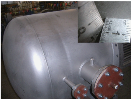
图1 管箱变形外观图 Fig.1 External view of the channel deformation
