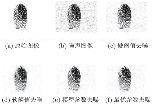
图 3 不同 \alpha 取值方法的去噪效果对比 Fig.3 The denoising effect comparison between processing methods with different values of \alpha
