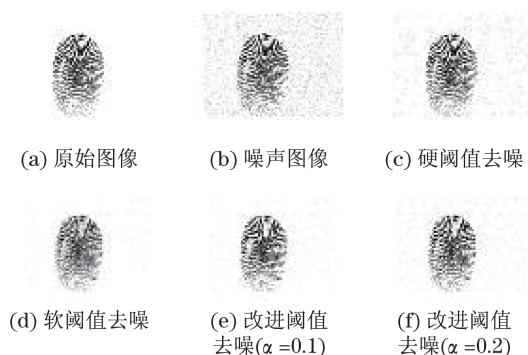
图 2 不同阈值函数的去噪效果对比 ( \alpha = 0.1 和 \alpha = 0.2 ) Fig.2 The denoising effect comparison between various threshold functions ( \alpha = 0.1 and \alpha = 0.2 )
