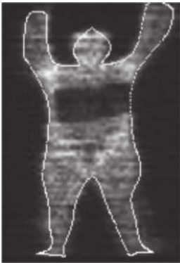
图 8 通过 ASM 模型提取的人体轮廓 Fig.8 Human body contour extracted by the ASM model
