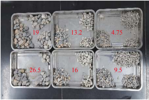
图 1 不同粒径的粒石化再生骨料 Fig.1 Different particle sizes of recycled aggregate
