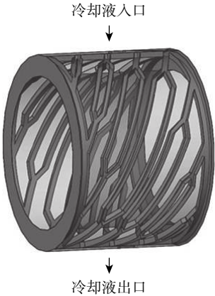
图4 昆虫翅脉仿生流道冷却结构示意图 Fig.4 Schematic diagram of channel cooling structure based on insect wing vein bionic
