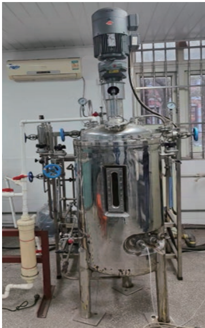
图1 实验装置结构图 Fig.1 Structure diagram of experimental device
