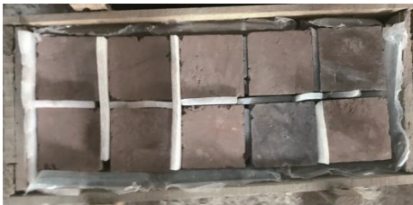
图 1 滇中红层泥岩岩样 Fig.1 Red mudstone rock samples from Central Yunnan
