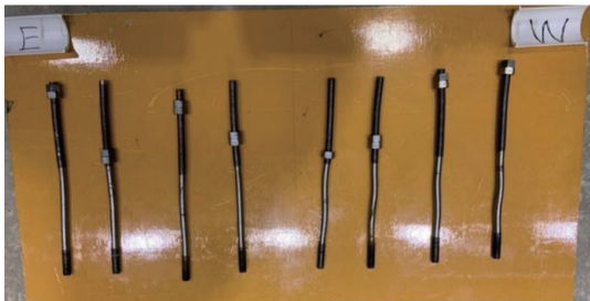
图9 UPLIFT3 阻尼器破坏情况 Fig.9 Damage in UPLIFT3 damper
