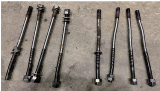
图8 UPLIFT2 阻尼器破坏情况 Fig.8 Damage in UPLIFT2 damper
